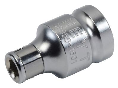
Hexagonal drive for accepting commercially available bits. With this adapter, 1/4" hexagon bits can be operated with cordless screwdrivers with 1/2" square drive. Chrome vanadium steel, chrome-plated finish with retaining ball. Particularly suitable for drywallers, carpenters, roofers and garden landscaping.
