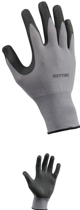
CE/EN 388-4131. Made of breathable, sturdy nylon material. Palms coated with nitrile foam. Excellent fit. Very good sense of touch. Providing good grip under humid working conditions. Excellent resistance to oil and grease
