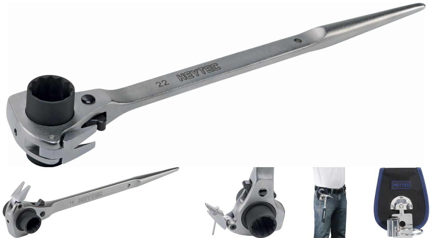
Chrome-Vanadium, chromium plated. This scaffolding ratchet-tool is an extremely robust product with reversible ratchet and pass-through feature for threaded bolts. With integrated fold-out nail puller. With rat-tail handle for aligning construction parts.
