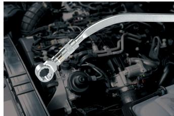
Chrome-Vanadium, C = chromium plated, For releasing the automatic tensioning device, Easy replacement of the belt, Also suitable for places with difficult access, High lever transmission for low effort, Form and force-fitting locking device for secure maintaining of the tool, Tools with metric- and Torx-wrench sizes for multiple applications
