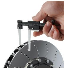
For measuring the thickness of built-in braking discs of passenger cars and motorbikes, made of stainless steel, with locking screw and additional tyre profile-calliper, Measuring range: 0-60 mm
