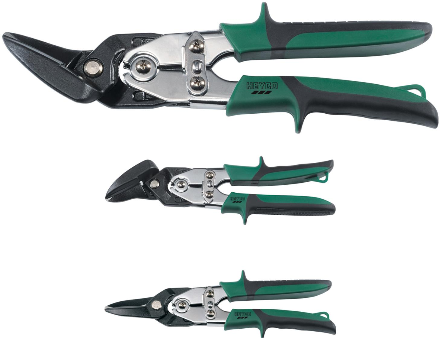
Universal tinmens' snips, BI = gun-metal finish, plastic-insulation with slip guard spring-loaded for automatic opening, Chrome Molybdenum Steel, phosphated, HRC 60-62, Cutting capacity: Metal up to 1,5 mm, Stainless up to zu 0,9 mm 1621-1 right hand cutting 1621-2 left hand cutting 1621-3 straight
