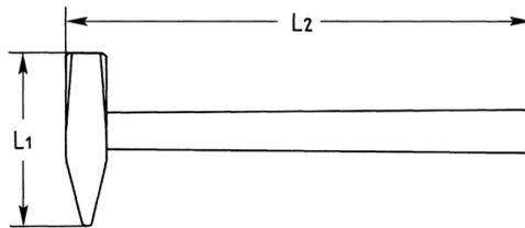
ST = standard, housing is partially filled with steel shot, which adds, to the weight, prevents rebound and provides “dead blows“ of maximum impact, replaceable nylon heads, hickory handle
