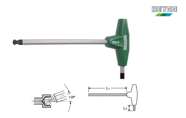
Chrome-Vanadium, C = chromium plated (with black tip) with shockproof plastic handle, spherical head permits usage on hexagon socket, screws located in confined or hard to reach areas off-axis operation up to 20°
