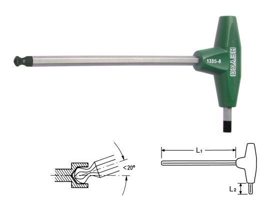
Chrome-Vanadium, C = chromium plated (with black tip) with shockproof plastic handle, spherical head permits usage on hexagon socket, screws located in confined or hard to reach areas off-axis operation up to 20°
