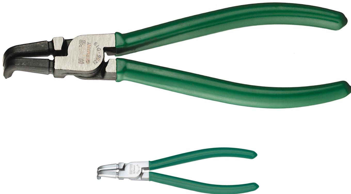
DIN 5256 D, Chrome-Vanadium, ASD = black, joint area polished, plastic coated handles, CPD = chromium plated, joint area polished, plastic coated handles, with bent jaws, black points, for internal circlips (bore holes) to DIN 472 + 984
