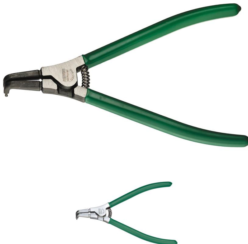
DIN 5254 B, Chrome-Vanadium, ASD = black, joint area polished, plastic coated handles, CPD = chromium plated, joint area polished, plastic coated handles, with bent jaws, black points, for external circlips (shafts) to DIN 471 + 983
