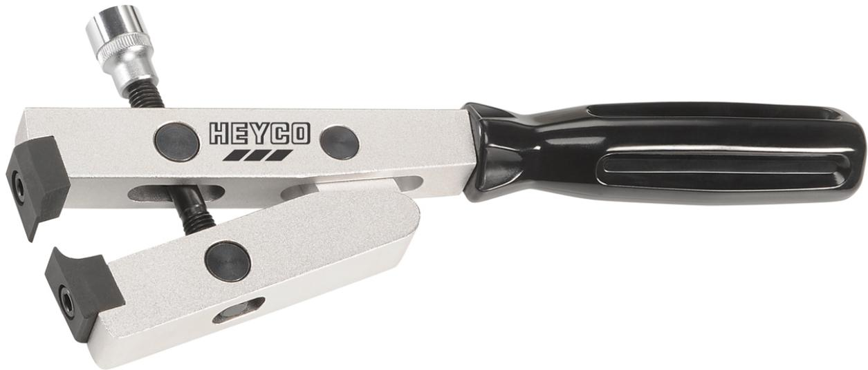
For clamping of fastener straps of axle collars and hoses, suitable for steel- and stainless steel-clamps, optimized weight through high-tensile aircraft aluminium, hardened clamping jaws, simple setting of the required torque through the 3/8" - drive by means of torque wrench, handle made of easily washable plastic, max. opening width: 45 mm, max. 30 Nm tightening torque Torque Wrench mandatory (otherwise breakage)
