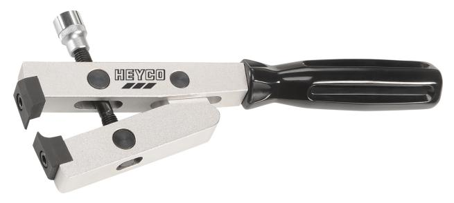
For clamping of fastener straps of axle collars and hoses, suitable for steel- and stainless steel-clamps, optimized weight through high-tensile aircraft aluminium, hardened clamping jaws, simple setting of the required torque through the 3/8" - drive by means of torque wrench, handle made of easily washable plastic, max. opening width: 45 mm, max. 30 Nm tightening torque Torque Wrench mandatory (otherwise breakage)
