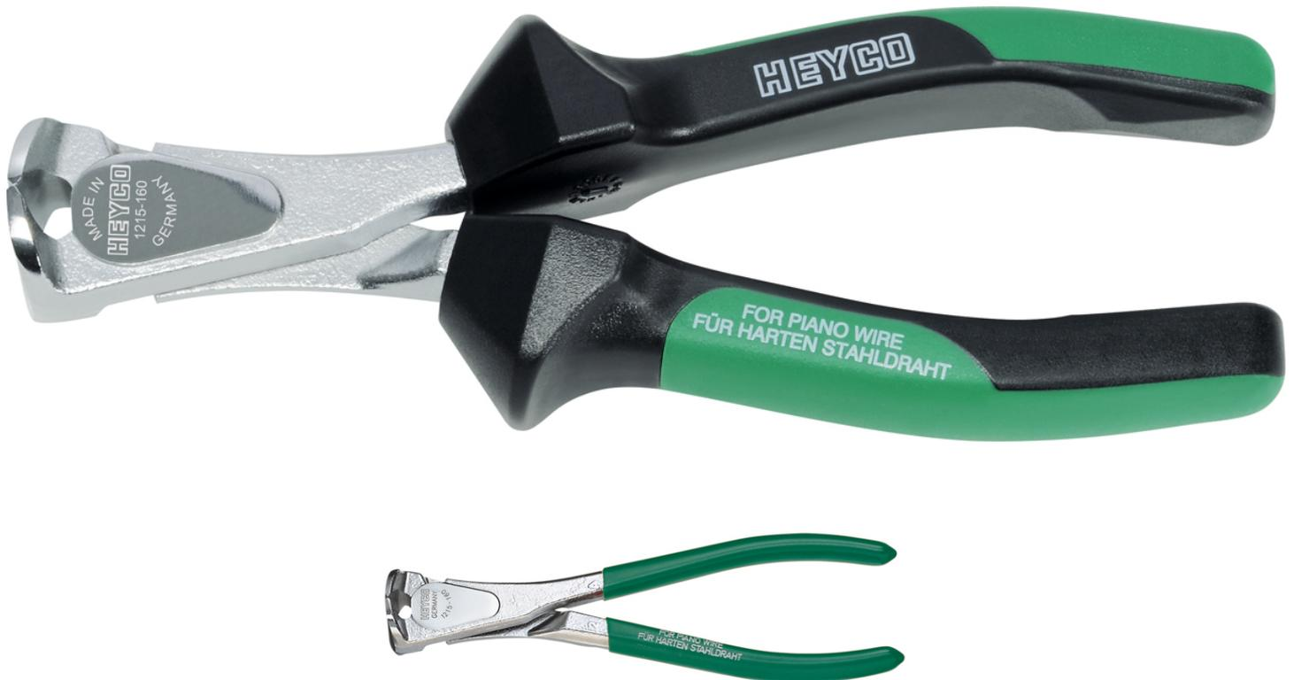
DIN ISO 5748, Special steel, CPD = chromium plated, polished head, plastic coated handles, CPI = chromium plated, polished head, formel plus plastic handle, with slip guard, cutting edges additionally induction hardened, for piano wire
