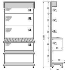
L = lacquered (scratch- and shock resistant plastic coating) made of 1,25 mm thick sheet steel, round hole perforation, 5 individual hang on boards 1000 x 400 mm for easy assembly, 4 of which are perforated, 3 plain shelves, 1 set of sub-divisions consisting of front- and rear division rails, 20 partitions and rail for price tags for middle or upper shelf, middle and upper shelf can be tilted, with adjustable pedestal and illumination.
