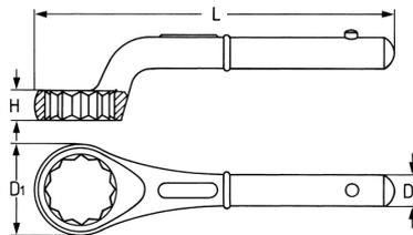
Chrome-Vanadium, C = chromium plated, heavy duty pattern, offset, to be used with tubular handles HEYCO 845
