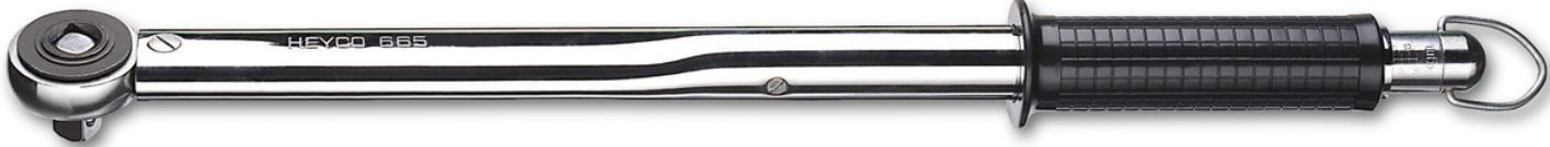
30 teeth · CPP = chromium plated, fully polished, with built-in push-thru ratchet for right and left hand threads, setting with knurled knob at end of handle, automatic release with audible and tactile signal when set torque is reached. Release accuracy  $\pm 4\%$
