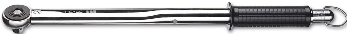
30 teeth · CPP = chromium plated, fully polished, with built-in push-thru ratchet for right and left hand threads, setting with knurled knob at end of handle, automatic release with audible and tactile signal when set torque is reached. Release accuracy  $\pm 4\%$
