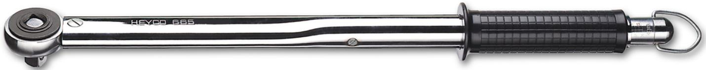
30 teeth · torque range: Nm 15–70, kpm 1,5–7, ft./lbs. 10–50, CPP = chromium plated, fully polished, with built-in push-thru ratchet for right and left hand threads, setting with knurled knob at end of handle, automatic release with audible and tactile signal when set torque is reached. Release accuracy  $\pm 4\%$
